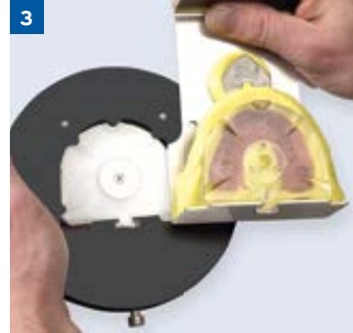
3 With the Giroform base plate inserted, the impression carrier is attached to the plate holder
