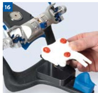
16 At the dental lab, the transfer table is placed in the articulator or the special mounting articulator used as a plastering device
